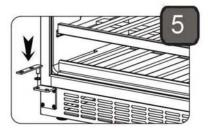
5. Install the lower hinge and bushing on the bottom left support bracket
